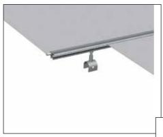
The HAKI Trak system consists of an aluminium alloy extruded track, which is fitted to the top chord of the HAKITEC 750 lattice beam with track clamps which are secured with 12 mm spring pins.
