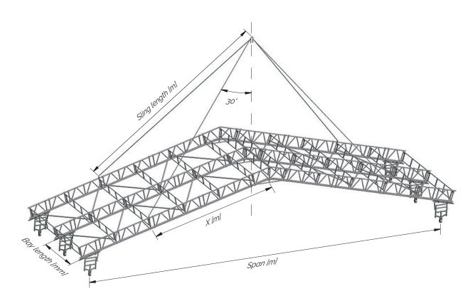
Lifting roof sections are an advantage when covering structures where supplies are to be provided by crane or when working on similarly shaped structures for which the covering can be moved from stage to stage. Weather protection roofs with a slope of 15° can usually be lifted in sections of 1-4 bays in length depending on the span (see tables 1-4). Sling lengths have been calculated for an angle of 30°.den (se tabell 1-4).
