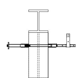
Place the HD Flange Clamp around the beam flange.
