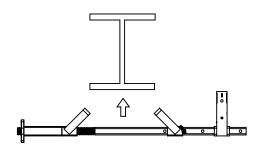
Loosen off wing nut to allow the HD Flange Clamp to fit over the I-Beam.
