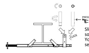
Slide the V-Post into the post socket on the HD Flange Clamp. You will hear a click when it is secured.
