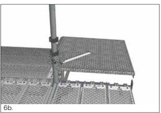
6. Lift the Corner Bracket and temporarily lock it a little higher on the standard.
