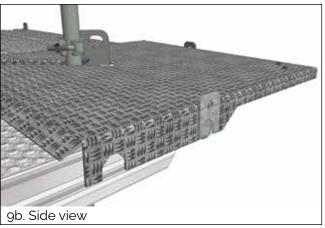
**9**. Lower the Corner Bracket into place, making sure that the cutout in the corner plate is fitted onto the Adjustable 2-3 Board Bracket. Lock the Corner Bracket.
