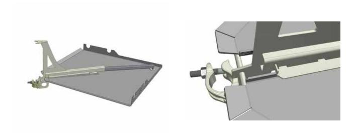
5. Insert the inner tube into the outer tube. Make sure the axle is under the plate at this stage.
