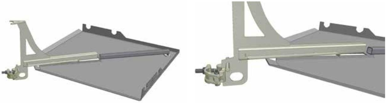
**3.** Bring the outer tube in the Bracket towards the inner tube on the Corner plate.
