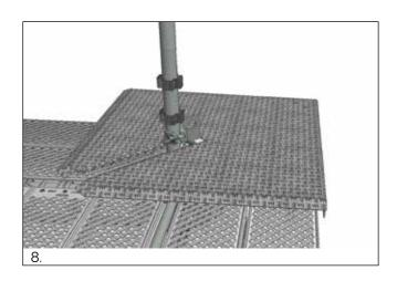
**8.** Slide the Corner Bracket in to its innermost position.
