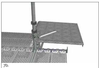
7. Dismantle the outer planks and retract the telescopic tubes of the Adjustable 2-3 Board Bracket.
