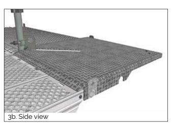
**3**. Lower the Corner Bracket into place, making sure that the cutout in the corner plate is fitted over the telescopic tubes of the Adjustable 2-3 Board Bracket
