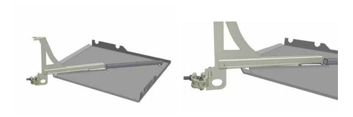
3. Bring the outer tube in the Bracket towards the inner tube on the Corner plate.
