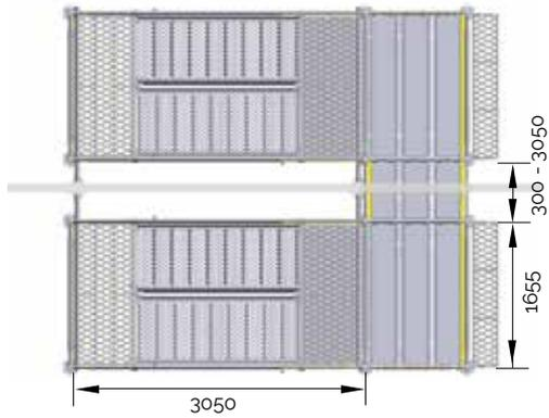
HAKI Stair Tower connected to another stair tower on the inside of the building
