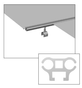
The HAKI Trak system consists of an aluminium alloy extruded track, with integral slots each side, fitted to the top chord of the HAKITEC750 beams with saddles secured by Spring Pins.
