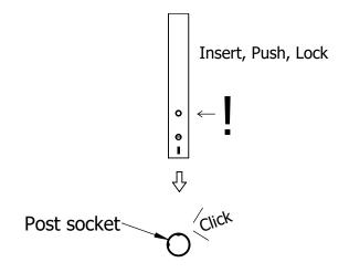
3. To remove the V-Post press the button near the bottom of the V-Post and pull in a upward direction.
