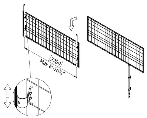
Move the sliders down to hook around the wire mesh of the barrier.
