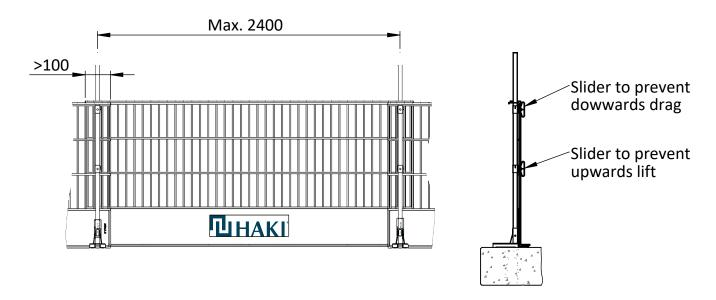
5. Class C barrier arrangements Note: MUST use Class C attachments and posts
