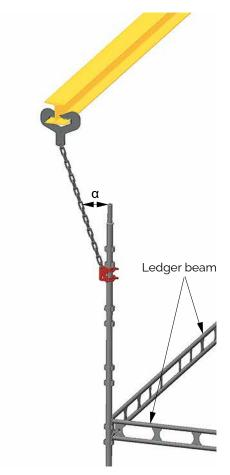
The Suspencion device must always be mounted directly below a group of pockets to avoid sliding.
