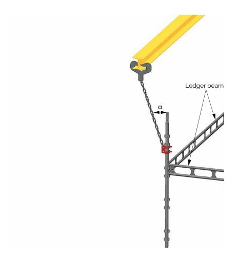
The Suspencion device must always be mounted directly below a group of pockets to avoid sliding.
