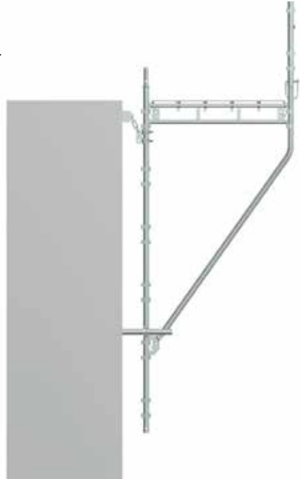
Example of suspended scaffolding with brackets.
