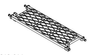
**V212-014**Stairway - Standard step handrail
