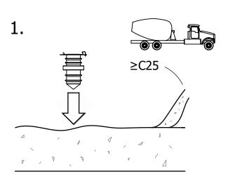
V-Cast must be used with C25 Conrete equivilant or greater.
