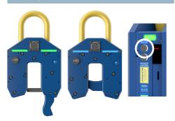
With the "Always On" mode, the colour code scheme of the LED status indicator will always be visible. Blue – for closed – and green – for open – are continuous for 10 seconds and then take an intermittent pattern in order to save battery. Activate this mode by pushing the top button beside the battery.
