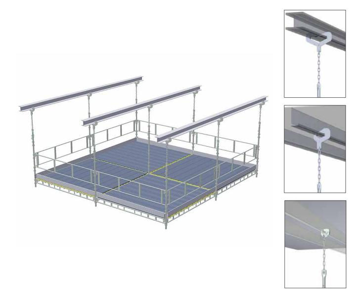
**HAKI Suspension devices** make it possible to suspend scaffolding from virtually any load-bearing structure.
