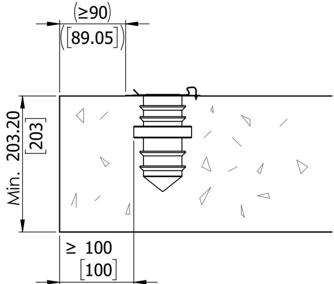
2. Allow concrete to sufficiently cure before removing the cap from the V-Cast and installing V-Posts.
