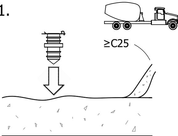
V-Cast must be used with C25 Concrete equivalent or greater.
